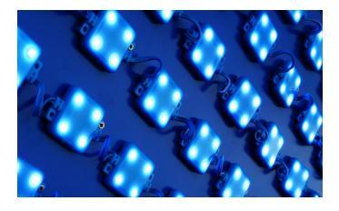
Over time, pixel pitch has become greatly reduced, meaning the spacing between lights has gotten shorter. This allows images to remain crisp and bright. Early LED signs were characterized by a pixel pitch of about 24mm, which was reduced to 20mm not too long afterward. This evolution then led to 16mm, then the current 10mm standard.
